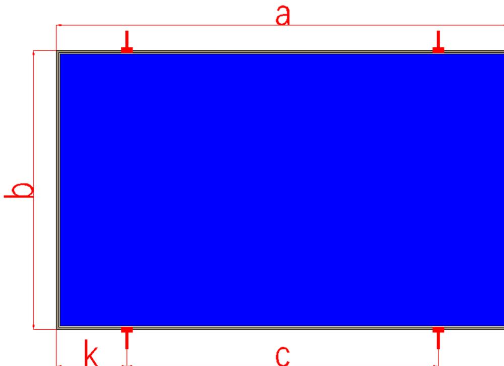
2. Install module with clamps at long sides of frames 2.在组件的长边用压块安装组件
