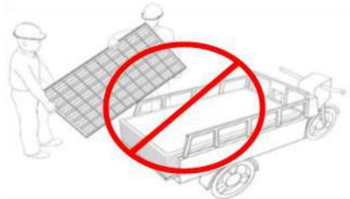
3.3.5 Do not transport the module with rope as shown below.
