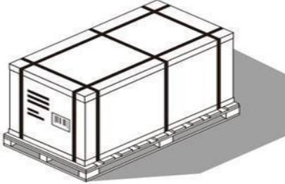
3.3.2 Packaged products can be transported by land, sea or air. During transportation, make sure that the package is fixed securely to the shipping platform without movement. Do not Stack more than two layers on truck.
