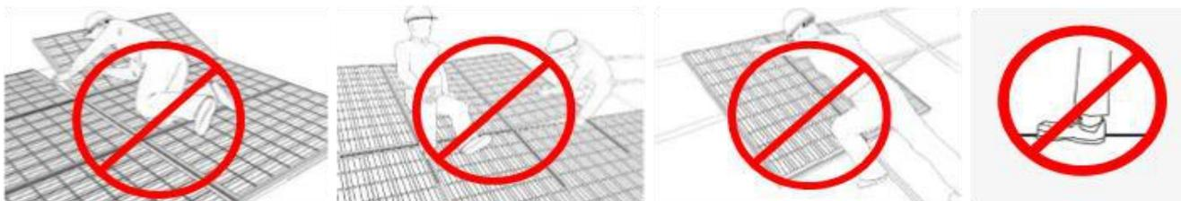
(2) Do not damage or scratch the front or backside surfaces of the module.
