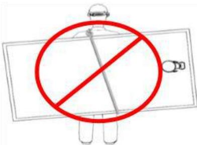
3.3.6 Do not carry the modules on the back of one person as shown below.
