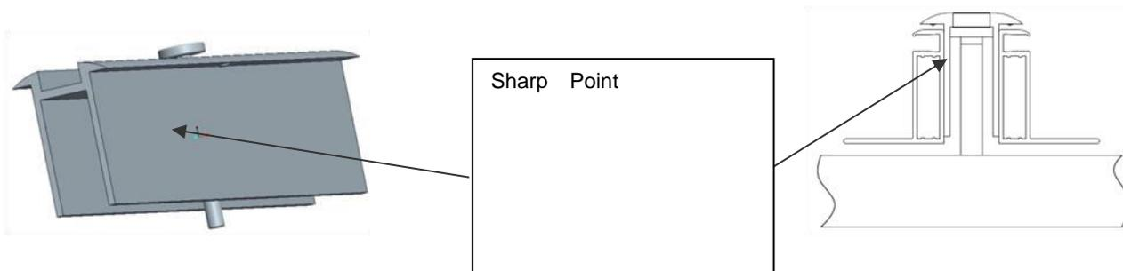
Recommended torque is 20.5Nm
