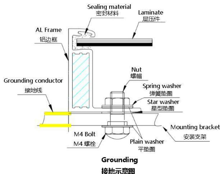
When grounding, each module can be grounded directly or in series or in parallel. If you choose the latter two options, it is recommended that the maximum number of modules connected in parallel should not exceed four, and in series should not exceed eight.
