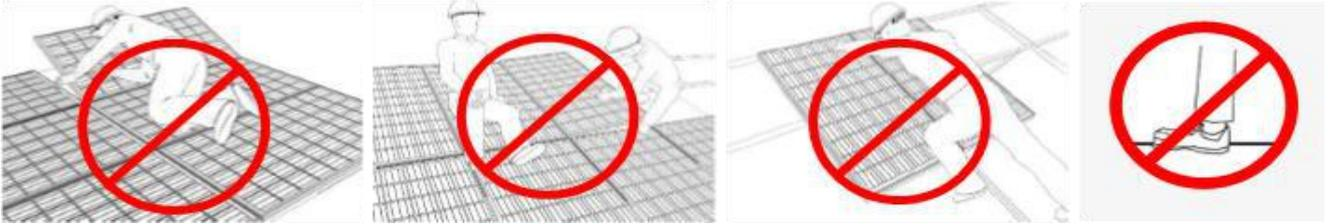
(2) Do not damage or scratch the front or backside surfaces of the module.
